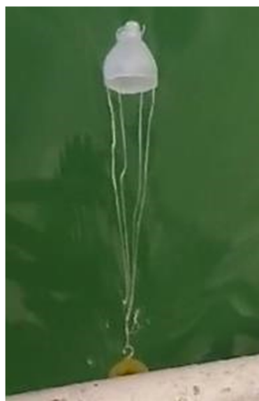
Fig. 4. Floating anchor No. 2 with 5 kg load cell connected
