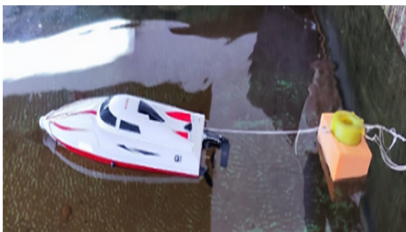
Fig. 3. Determination of the force of thrust on the moorings of the boat model under test
